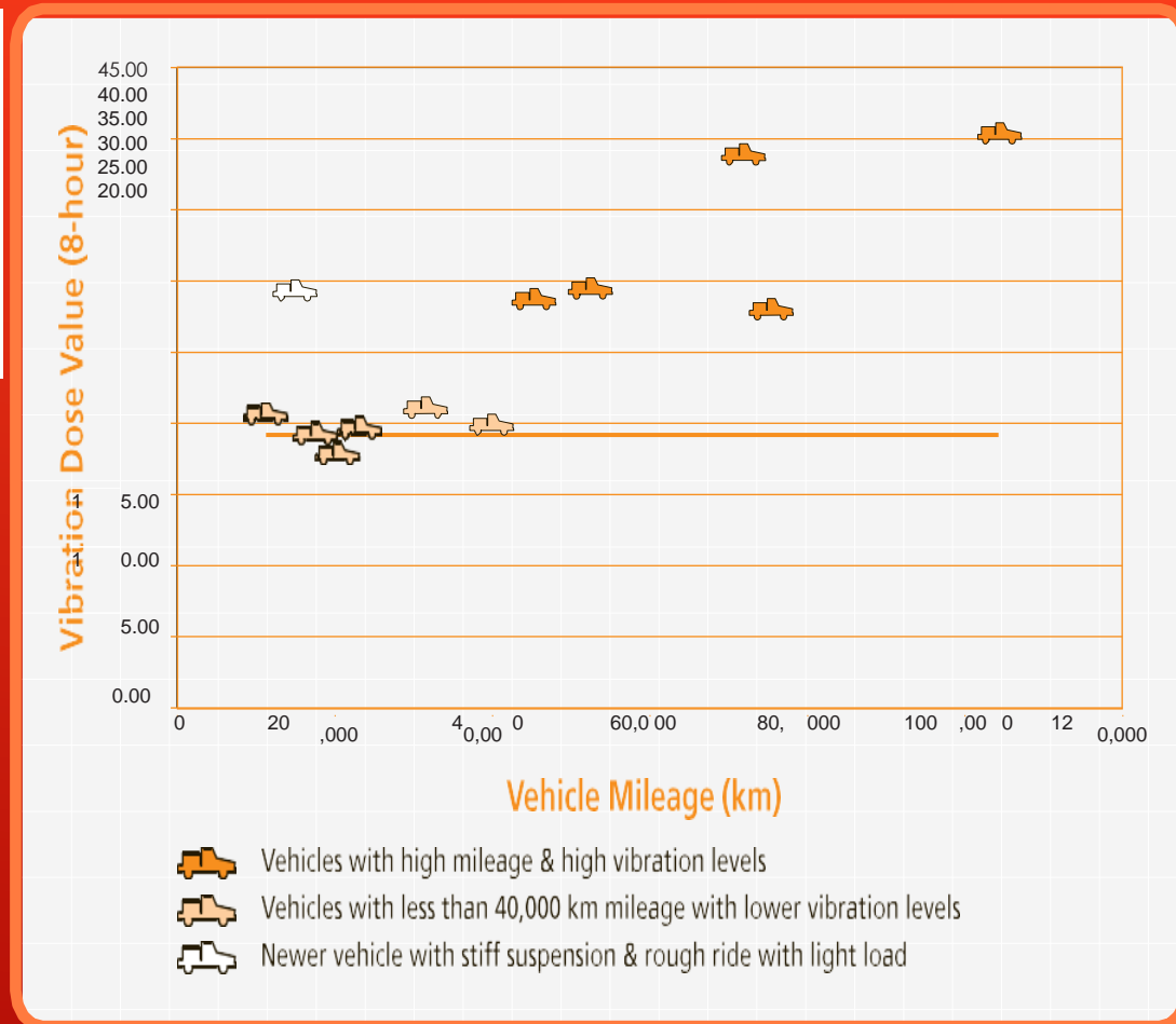
FIGURE 3: Vehicle mileage versus ride roughness. Higher VDV means rougher ride. See Section 3 for explanation of Vibration Dose Value (VDV).
